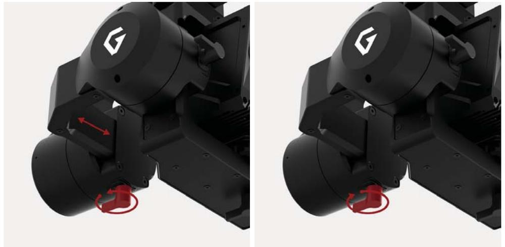
1. Loosen the thumb screw underneath the roll bar, then gently slide the roll bar left or right until roll axis remains level.
