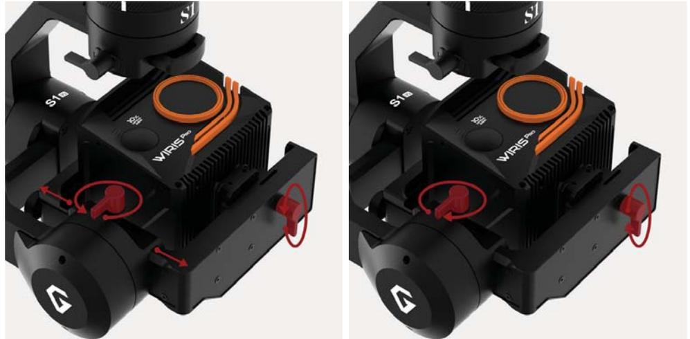
1. Rotate the tilt axis so that the lens is pointing upward. Then, loosen vertical adjustment thumb screw, gently slide the camera mount crossbar and the top bar forward and backward until the camera remains pointing upward when released.
