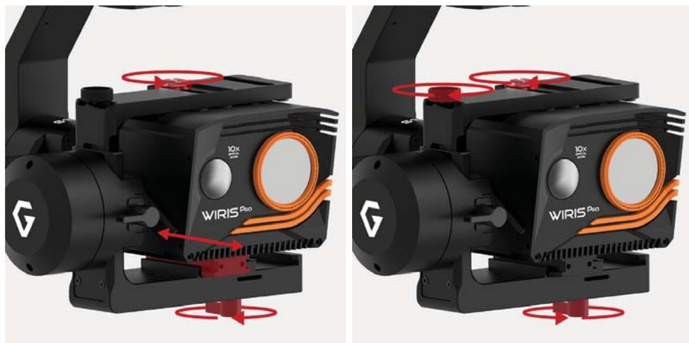
1. Loosen the thumb screw underneath the camera plate and the top bar screw. Then, gently slide the camera forward or backward until the tilt axis remains level.
