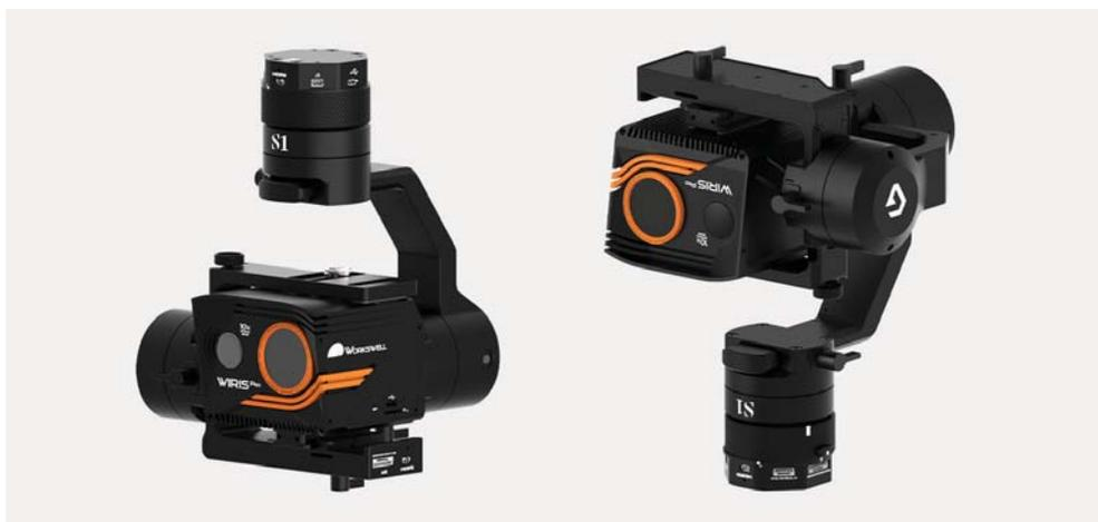
After powering up the gimbal , it will automatically detect if the gimbal is in inverted operation or normal operation based on pan motor position.
